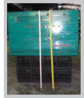
Creep testing on the Heavy Duty R-Tank (5-Plate) was done using four Double R-Tanks, also unconfined.
